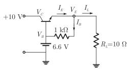
We can analyze that the transistor is operating in active region.
