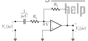
$$\frac{0 - V_i(j\omega)}{\frac{1}{j\omega C} + R_1} + \frac{0 - V_o(j\omega)}{R_2} = 0$$
