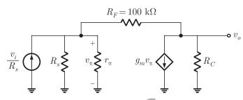
This is a shunt-shunt feedback amplifier. Given parameters,
