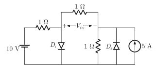
In the above circuit diode  $D_1$  must be ON, as it is connected with 10 V battery now the circuit is
