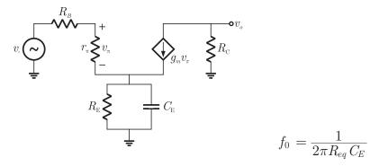
$\operatorname{Req} \rightarrow \operatorname{Equivalent}$  resistance seen through capacitor  $C_E$
