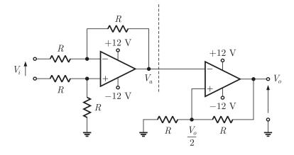
The first half of the circuit is a differential amplifier (negative feedback)  $V_a = - (V_i)$
