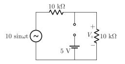
Output voltage  $V_0 = \frac{10\sin\omega t}{10+10} \times 10 = 5\sin\omega t$
