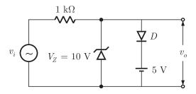
Assuming forward voltage drops of the diodes to be 0.7 V, the input-output transfer characteristics of the circuit is
