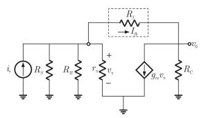
Here the feedback circuit samples the output voltage and produces a feed back current  $I_{fb}$  which is in shunt with input signal. So this is a shunt-shunt feedback configuration.
