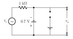
The output  $v_o = -0.7 \text{ V}$ 2. When  $-0.7 < v_i \le 5.7$ , both zener and diode *D* will be off. The circuit is
