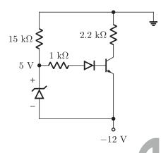
We can see that both BE and BC Junction are forwarded biased. So the BJT is operating in saturation.
