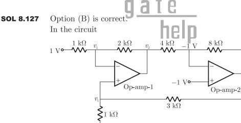
Writing node equation in the circuit at the negative terminal of op amp-1
