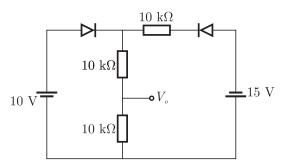
We can observe that diode  $D_2$  is always off, whether  $D_1$ , is on or off. So equivalent circuit is.
