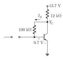
Using KVL in input loop,
