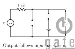
Note that zener goes in reverse breakdown(i.e acts as a constant battery) only when difference between its p-n junction voltages exceeds 10 V. 3. When  $v_i > 5.7$  V, the diode D will be forward biased and zener remains off, the equivalent circuit is
