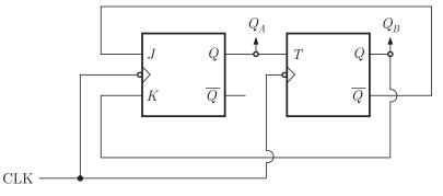
It the state  $Q_A Q_B$  of the counter at the clock time  $t_n$  is '10' then the state  $Q_A Q_B$  of the counter at  $t_n + 3$  (after three clock cycles) will be (A) 00 (B) 01
