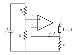
Since op-amp is ideal  $v_+ = v_- = v_1$ Writing node equation.
